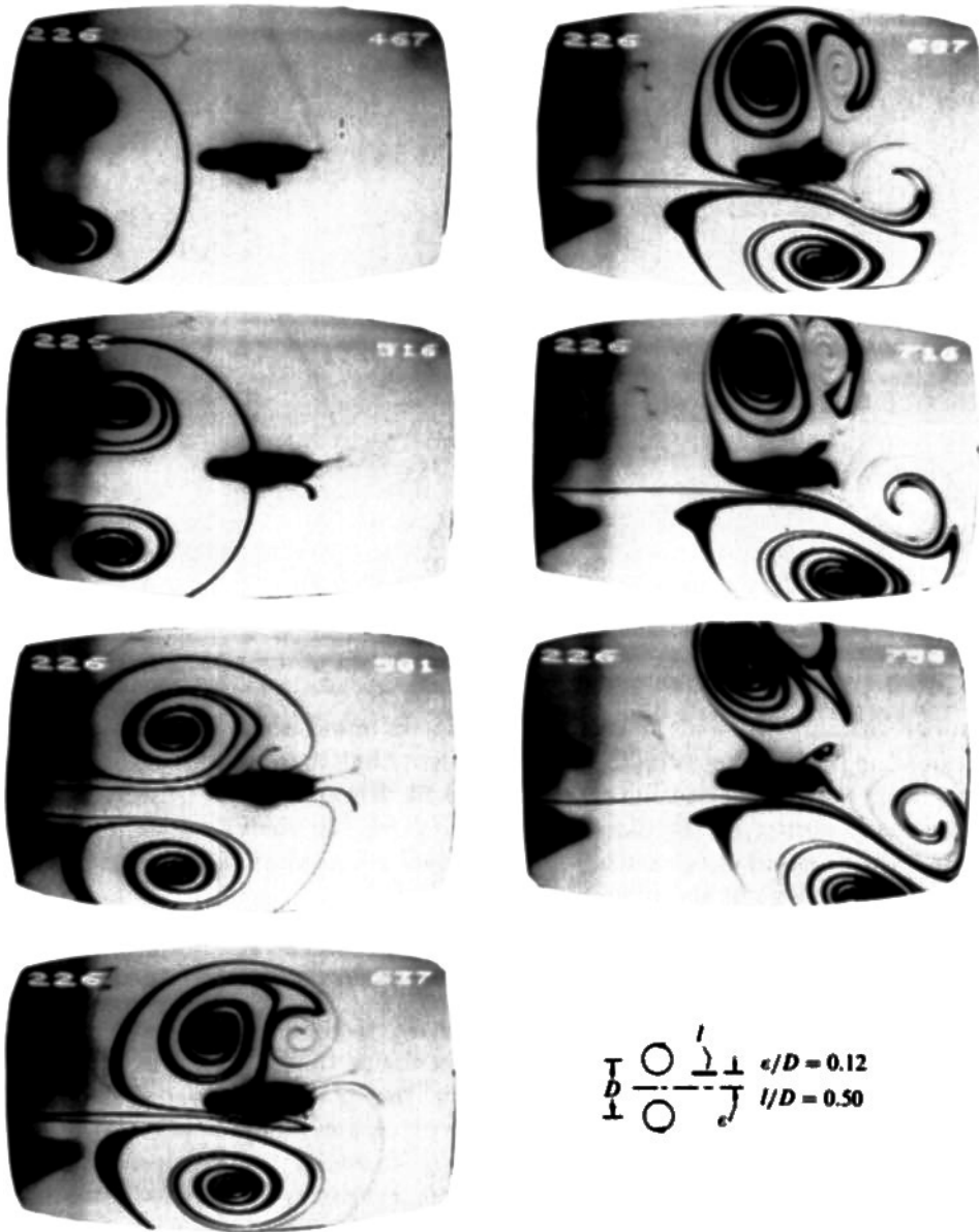
FIGURE 13. Antisymmetrical mode of secondary vortex formation from plate slightly displaced from centreline of incident vortex pair; \epsilon/D = 0.12 , l/D = 0.50 .
